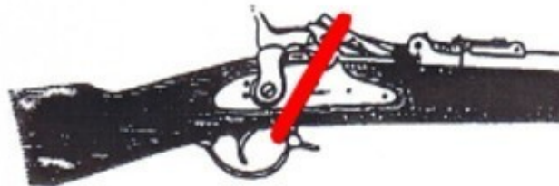
Hammer Down, Trap Door Partly Open Tied Down on Hammer
